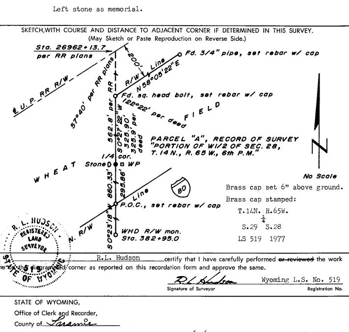
This "corner record" was filed for record on the 9 day of 40. on the cross-index plat and is assigned page No.\_\_\_\_, in book No.\_\_\_\_
